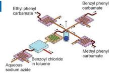
All for one and one for all: A continuous-flow, multistep microchemical synthesis of carbamates starting from aqueous azide and organic azoyl chloride by using the Curtius rearrangement reaction is described. The procedure involves three reaction steps and two separation steps (one gas—liquid and one liquid—liquid). Formation of a microreactor network for parallel synthesis of analogous compounds is also demonstrated.
