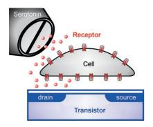
An unlike pair: A serotonin receptor is functionally coupled to a silicon chip by means of cell-transistor interfacing. The transistor signal is proportional to the membrane cell current of activated receptors. The development of this receptor-cell-transistor biosensor provides the physicochemical basis for noninvasive drug screening.
