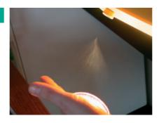
Weaving webs: Electrospinning is a highly versatile method for the preparation of polymer and metal nanofibers. Fibers with complex morphologies or specific functions for various applications (for example, filtration, textiles, sensors, optics, catalysis, drug delivery, wound dressings, tissue engineering, and plant protection) can be designed through the selection of suitable systems.
