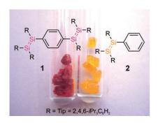
Electronic communication between two Si-Si double bonds is enabled by a phenylene linkage and expressed in a large red shift of the longest-wavelength UV/Vis absorptions of deep red tetrasiladiene 1 compared to yellow phenyldisilene
