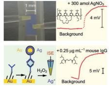
Pushing the limits: A silent revolution of ion-selective electrodes (ISEs) took place during the past decade. Polymeric membrane electrodes are now routinely used to determine complex formation constants between lipophilic guests and ionic hosts. Ultratrace level measurements have become possible even in samples of very small volumes, with detection limits in the attomole range.
