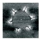
distinctive patterns. The resulting STM image (see picture, right) shows a triangular region of reduced hydrogen concentration surrounded by white features due to subsurface hydrogen.
